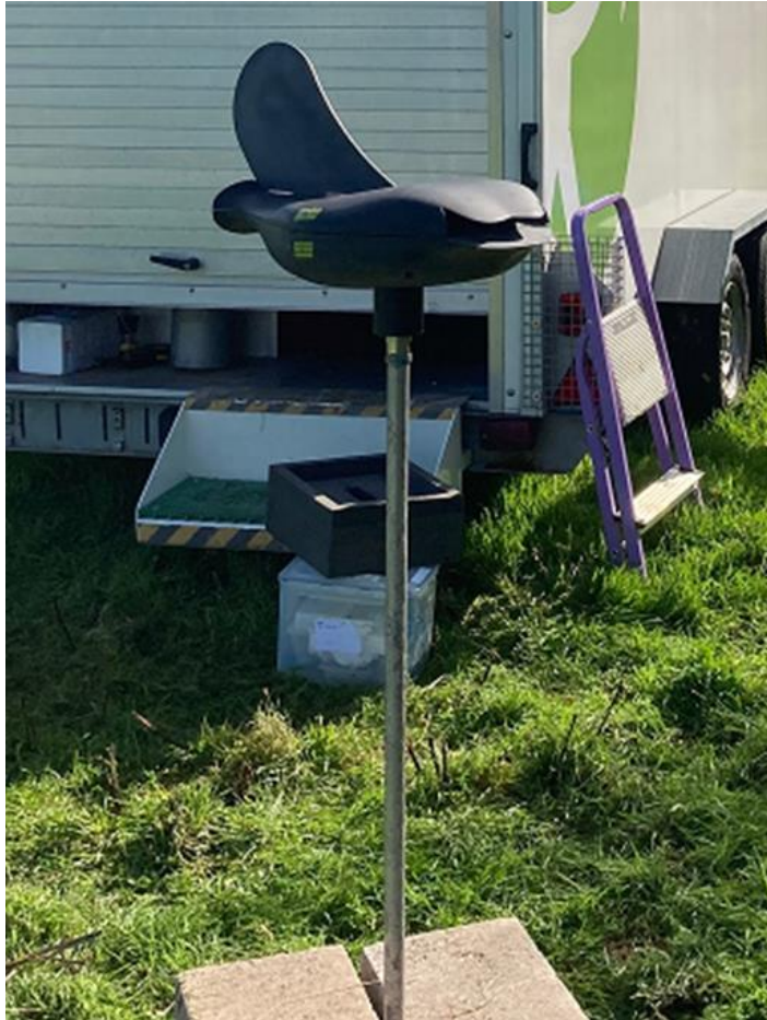
Figure 1. DPAS showing inlet to airway and vane that turns it to face upwind. The inlet is ~1.3 m above ground.
